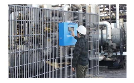
Scentinal is easy to setup and use. Each Scentinal comes pre-loaded with a SIM card so all you have to do is mount it to a wall or a pole and power the unit up. Scentinal will detect its location using built-in GPS, and start transmitting to the central server. All configuration and maintenance can be done on the on-unit 7" touch screen monitor or remotely through the SIMS software. (To know more about SIMS software check page 17)
