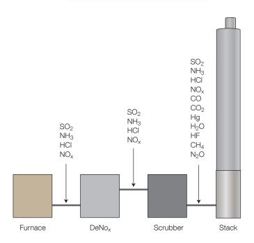
The OPSIS monitoring system is an effective tool for controlling the different emissions and process control spots in a bio plant.
