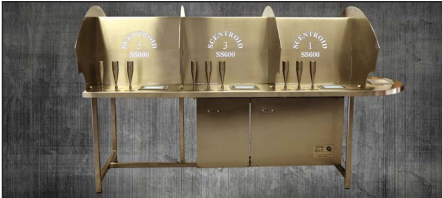
The Scentroid SS600 is industry's first olfactometer that uses high-accuracy Mass Flow Controllers to monitor and adjust both the sample air and the clean diluting air, ensuring accurate dilution ratio regardless of variations in ambient pressure or temperature.
