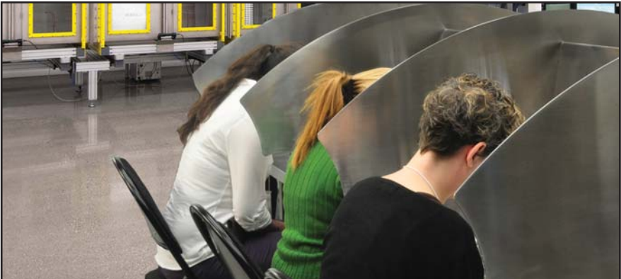
The Scentroid SS600 is the world's most advanced stationary, dynamic, and fully automated olfactometer. It is capable of odour measurement and analysis to all international olfactometry standards: EN13725:2003, ASTM E04-679, NVN2820, VDI 3881, GB/T93-14675, AS 4323.3
