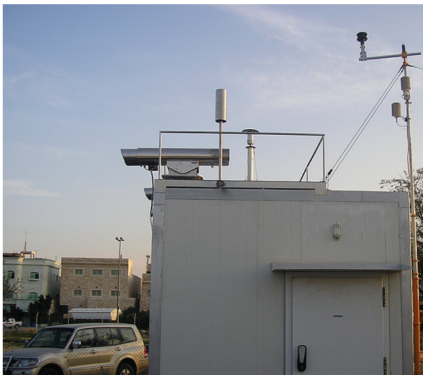
The OPSIS monitoring system is an important tool for continuous environmental control of a range of gaseous compounds at street level.
