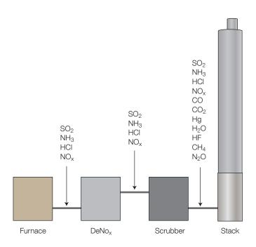
The OPSIS monitoring system is an effective tool for controlling the different emissions and process control spots in a waste incinerator
