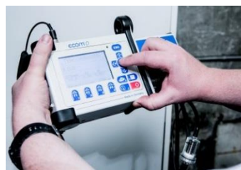
With length-adjustable holding strap. Can be fitted to the individual hand size thanks to Velcro strip.
