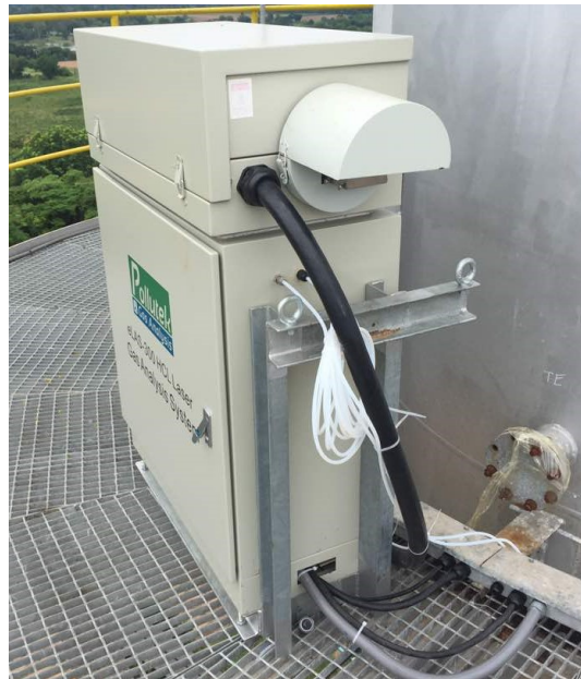
eLAS-300 in-situ extractive TDLAS Laser analysis system Hot Wet (HW) principle for NH 3 , HCl, HF or/and H 2 O. Other version: eLAS200-Probe in-situ extractive
