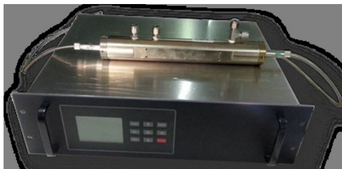
Hot wet analyzer design with external heated gas chamber
